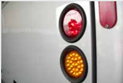
Exterior Lighting - All exterior lamps are to be replaced with new LED
