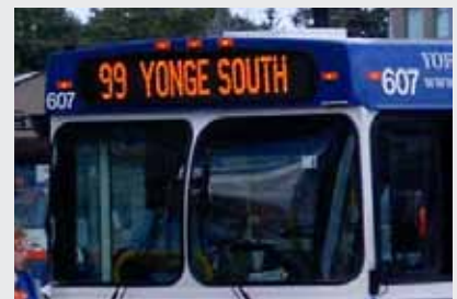
Destination Sign - New state of the art LED sign systems including front, side and rear destination signs assure ADA compliance
