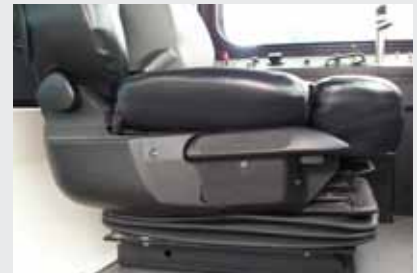
Seating - New driver's seat features state of the art air suspension systems with multiple adjustments for optimum driver comfort.
